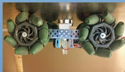
Figure 4: Close-up View of The Mounting System, August 2017. The magnets are mounted between the wheels to create an even distribution of the pull force on the wheels.
