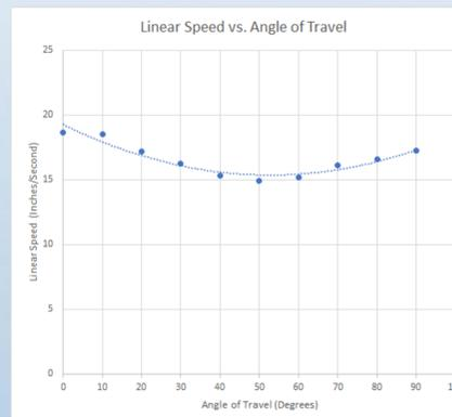
Figure 6: Data Collected to Determine the Relationship Between Angle of Travel and Linear Speed.
