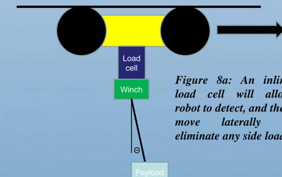
Figure 8a: An inline load cell will allow robot to detect, and then move laterally to eliminate any side loads
