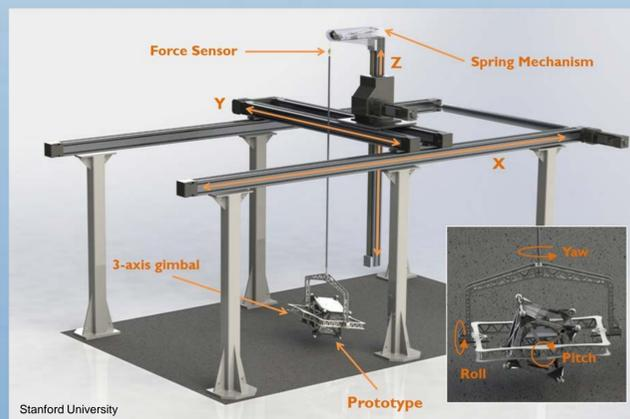
Figure 3: Prototype Gravity Offloading System for the Testing of Surface Mobility of Small Bodies. <https://asl.stanford.edu/projects/surface-mobility-on-small-bodies/>
