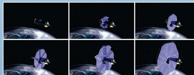
Computer-generated model of an in-space deployable solar array for solar electric power. (Zirbel, Lang, Trease, et al, JMD 2013)
