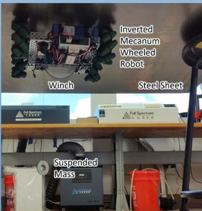
Figure 2: The Inverted Mecanum Robot, Tested August 2017. Testing of a prototype mecanum robot. Basic movement ability and magnetic inversion has been tested and verified.
