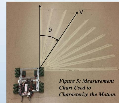
Figure 5: Measurement Chart Used to Characterize the Motion.
