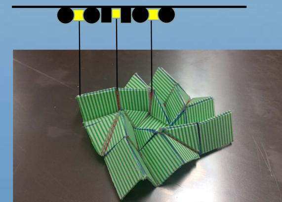
Figure 8b: Origami Flasher that Requires Multipoint (using multiple robots) Gravity Offloading.
